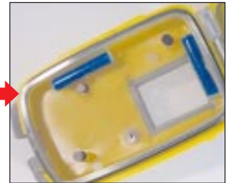
8. Insert Moisture Muncher drying agent to prevent fogging.
