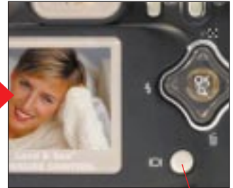
16. Push and hold the LCD button for 3 seconds to exit Quick Review.
