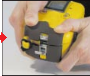
10. Close the housing tightly. Do this in a dry, air-conditioned room to prevent fogging.
