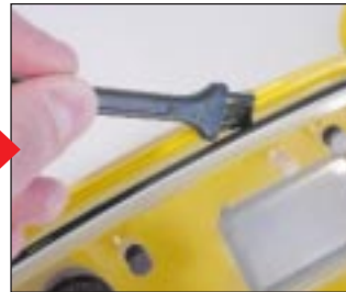
7. IMPORTANT: Clean O-ring with brush. Carefully inspect O-ring for cuts or damage.
