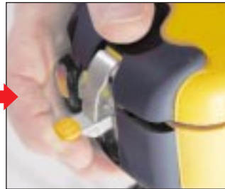
6. Open the housing. Use the tab under the latch. Keep lid pushed down to release the latch.
